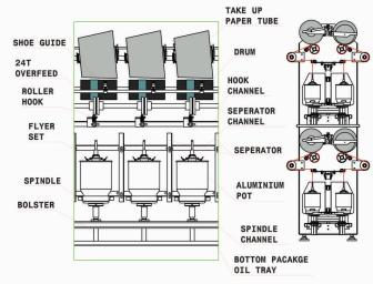
National SPUN TFO machine is the most Efficient choice, in terms of production cost, for producing 2ply-3ply & multiply doubling twisting of yarn like Spun yarns, Cotton Yarns, PC, PSF. PV, we have twisting solutions from (90MM - 310MM) spindle size and for almost any industry you can come up with.
