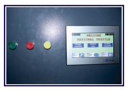
Plc system with touch screen HMI display to access and control machine working parameters effortlessly just with control of simple touch. Servo motor and servo systems ensures precise and steeples setting of all parameters.
