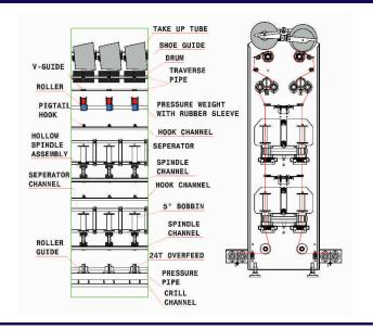
National Elastic yarn covering machine or rubber yarn covering machine, widely used for manufacturing yarns for making elastic tapes, face mask elastic, elastic string, garment elastic accessories, garment smoking, used in production for undergarments, socks panty hose, etc
