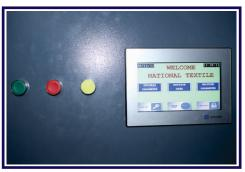
Plc system with touch screen HMI display to access and control machine working parameters effortlessly just with control of simple touch. Servo motor and servo systems ensures precise and steeples setting
